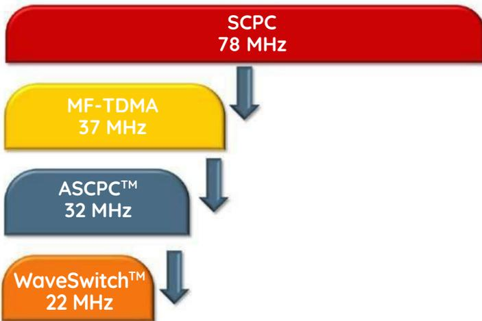
As we can clearly see below in the above and below diagrams, SCPC is the most inefficient waveform in terms of -statistical multiplexing factor and spectral resources expenditure while ASCPC™ demonstrates the best efficiency out of the three.
